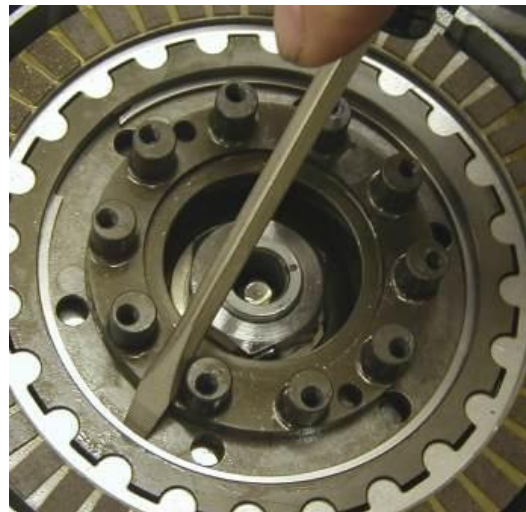
Use a screwdriver to ensure the ring is seated by sliding along the ring's inner diameter.
