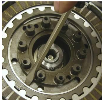
Threading retaining ring into groove
