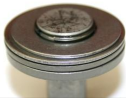
Rekluse washer snapped down into place over the throw-out clip
