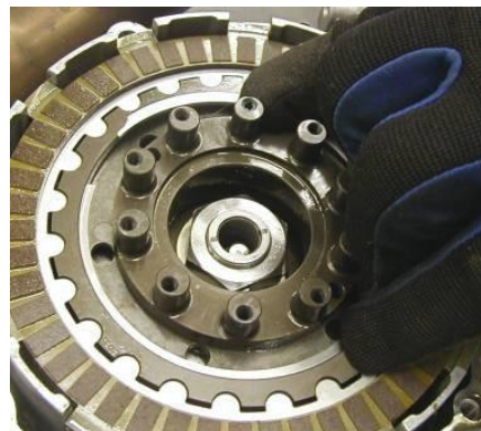
Threading retaining ring into groove
