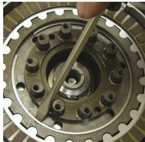
Threading retaining ring into groove
