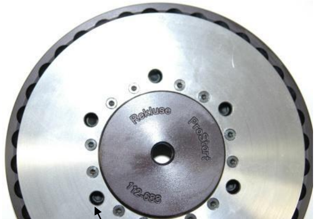
Screws lined up with access holes in the ProStart Top Plate
