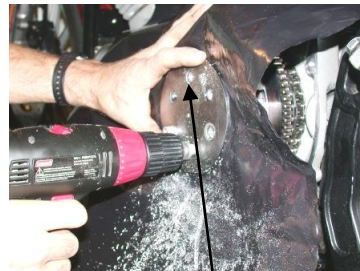
Maintain pressure against the guide plate so that it remains seated against the clutch hub, guaranteeing each stand-off is milled down equally.
