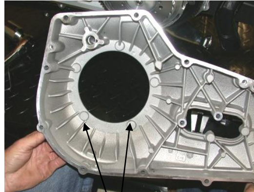
The 2 lower screw bosses that need to be modified
