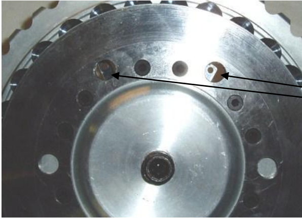
Retaining Ring Tabs lined up with access holes in the ProStart Top Plate
