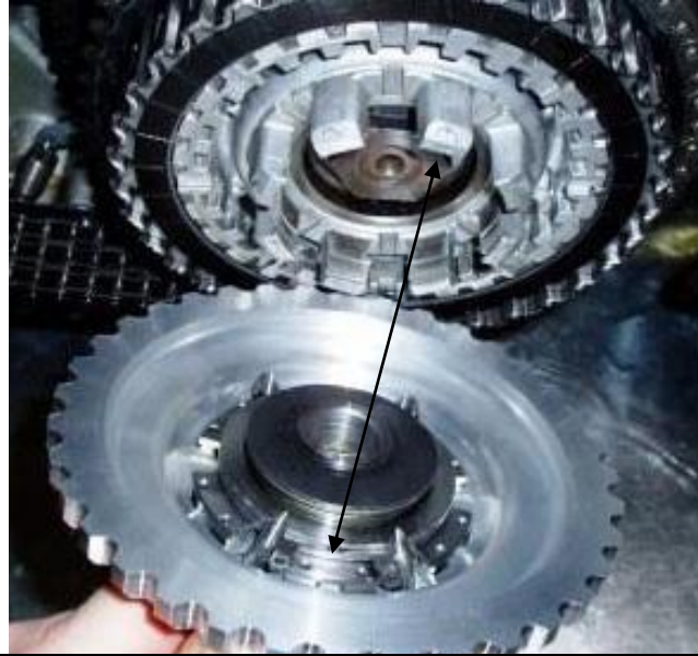
Gap between the 2 Retaining Ring tabs centered over one of the 8 center clutch posts.
