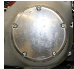
Bottom two Derby cover screws installed with one 6mm spacing washer added
