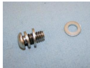
Derby cover screw with 6mm spacing washer added behind the head
