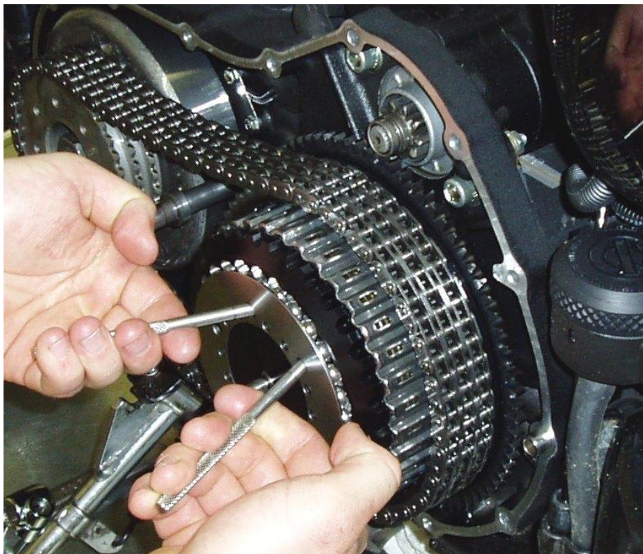
Gap between the 2 Retaining Ring tabs centered over one of the 8 center clutch posts.
